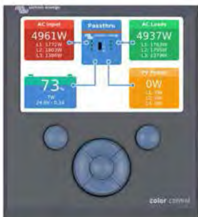
Color Control panel, showing a PV application
